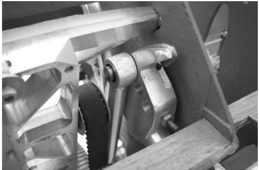
A view of the core flapping mechanism in the Reynolds ornithopter.
