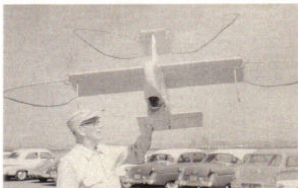
Percival Spencer holds the 70-inch-span, free-flight prototype of the ornithopter.
