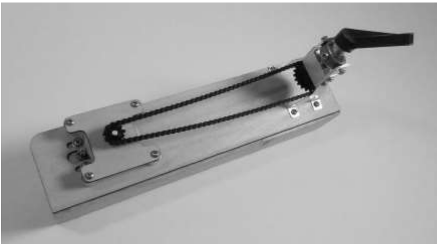
The author's reconstruction of the Schmid mechanism used an electric motor and a miniature plastic drive chain.
