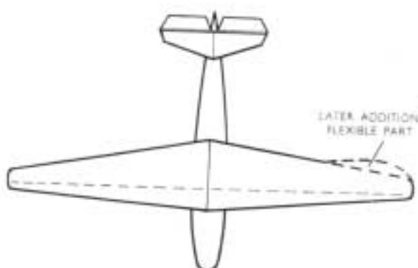
FIGURE 2. Sketch of the plan view of the "Schwinguin." The span was between 9-10 m.
